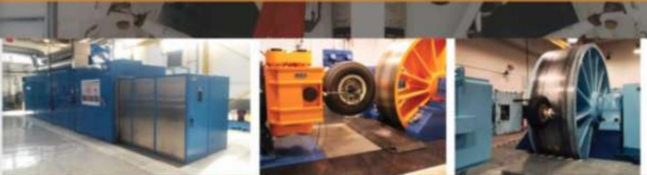
LINK's aircraft dynamometers simulate conventional and emergency braking conditions and landings at speeds up to 350 mph. Our roll dynamometers are utilized for testing of aircraft wheels for measuring performance of wheel designs. See below a snapshot of LINK aircraft testing solutions:
